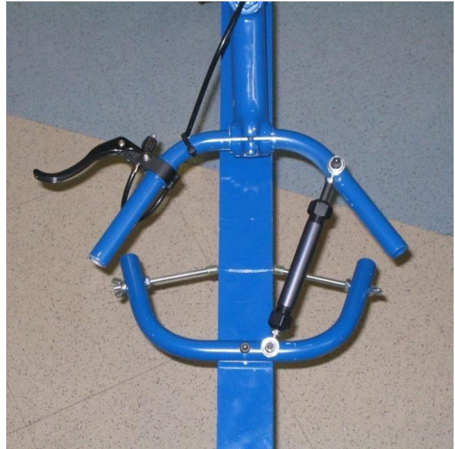
Fig. 14.18. The two handle bars connected with the compensator.
