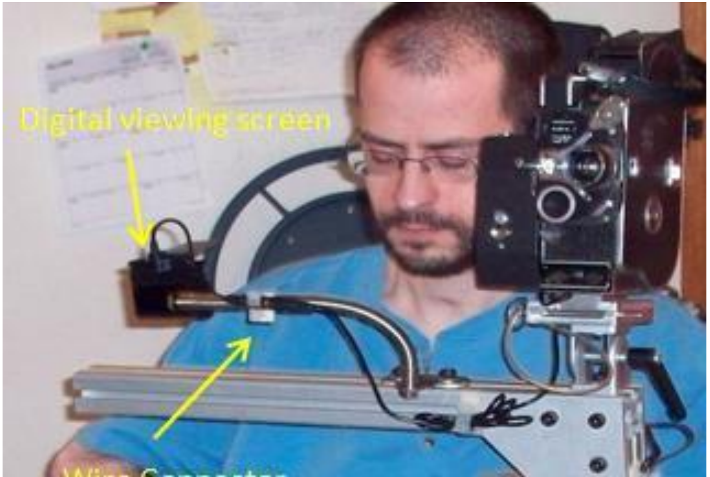
Fig. 14.9. Zigview remote viewing system.
